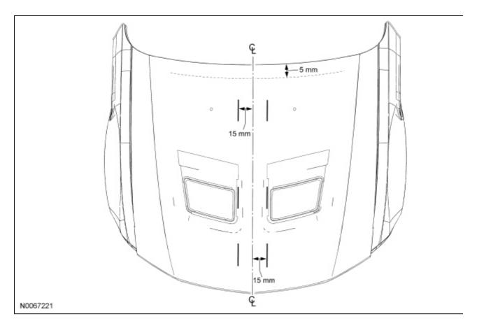
5. **NOTE:** Surface temperature of body panel(s) should be above 10℃ (50年). Avoid carrying out installation of stripe decal(s) in direct sunlight.
